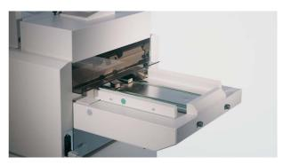
**Document Table** The inserts are fed to the document table from either the document feeder models Plockmatic 306/310/320 or manually. When manually fed, speed is automatically adjusted to the operator.
