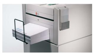
**Receiving Tray** The envelopes are counted and stacked on the receiving tray, ready to be franked and posted. Warning sensor notifies operator when the envelope stack needs to be emptied.
