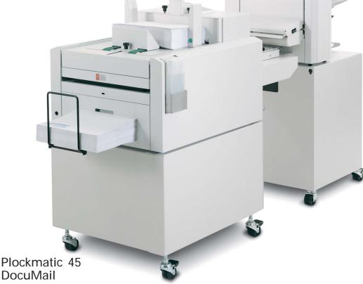
Extremely compact in size, no bigger than an ordinary copier and yet capable of 3600 inserts per hour and up to 12 mm inserting capacity. The operator friendly design with multilingual LCD display combined with microprocessor controlled settings and step-by-step guidance through the different menus, reduces set up time to less then 1 minute for a new job.
